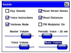
Press inside the box to the left of each feature to check it (turn on) and uncheck it (turn off).
